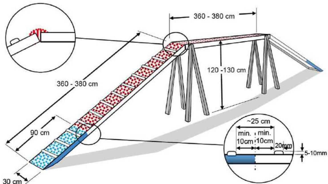
Height: minimum 120 cm – maximum 130 cm Plank and ramp length: minimum 360 cm – maximum 380 cm Plank and ramp width: 30 cm Contact areas: The last 90 cm from the bottom of each ramp must have a different colour. **Both the surface and the sides of the contact area should be in the same colour (along its full length).**
